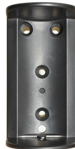
The vessel's cable can enter the bracket from the rear, side, or bottom by drilling or filing to the desired opening for any size cable. The bracket has a removable tab on the bottom if needed.
